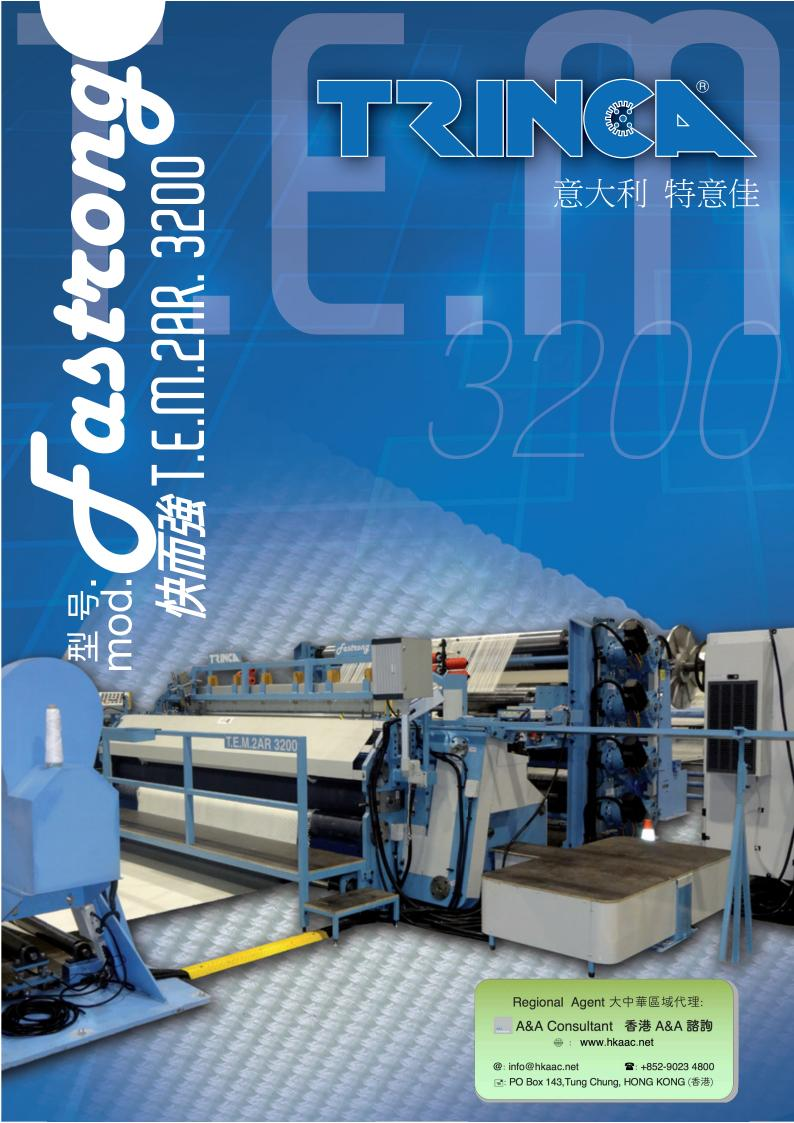
技术用布高速织机 • Fast weaving loom suitable to weave technical fabrics
